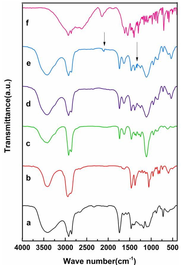
**Figure 2:** Fourier Transform Infrared FTIR Spectra of (a) Cholesterol, (b) Span™ 60, (c) Tween60, (d) Niosome, (f) Gabapentin loaded niosome (g) Gabapentin.
